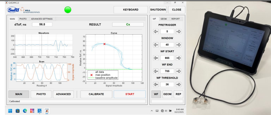
Cross-correlation for high precision T-o-F measurement
